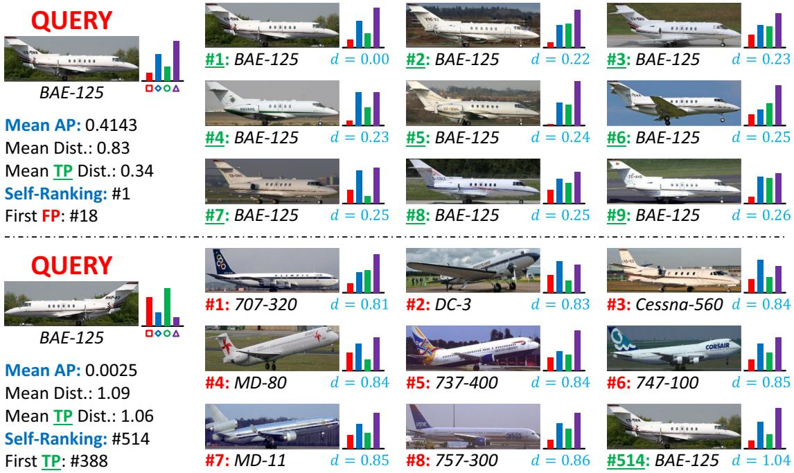
**Fig. 2** Content-based image retrieval on the right-oriented **Aircraft-100** dataset (best viewed in color). We use the same query image with different orientations. *AP* for average precision, *TP* for true-positive, *FP* for false-positive (Color figure online)
